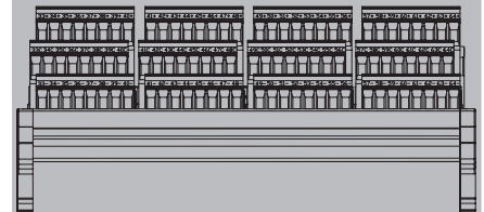
Field terminals view for ADV161 (Channels 33 to 64)
