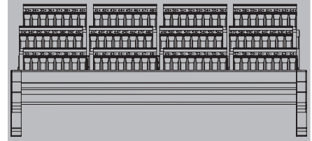
Field terminals view for ADV161 (Channels 33 to 64)
