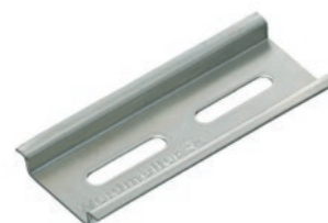
TS 15/5.5 mm according to EN 60715 (s = 1.0 mm)
