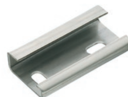
TS 32 mm according to EN 60715 (s = 1.5 mm)
