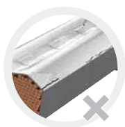
Formation of cracks at the impressions of the crimping jaw
