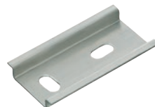
TS 35/7.5 mm according to EN 60715 (s = 1.0 mm)
