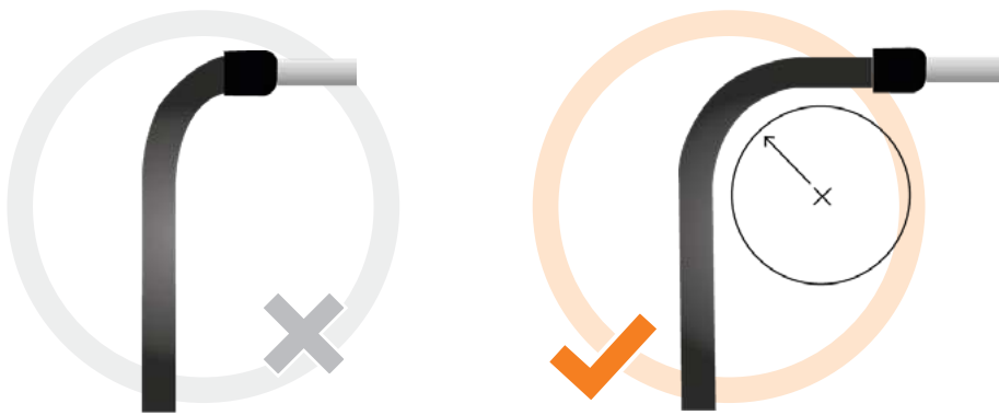
Risk of breakage due to overload
