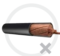
Pulled out conductor
