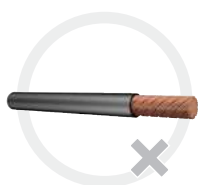
Excessively twisted individual wires
