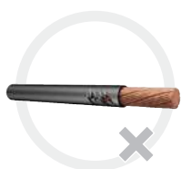
Damaged conductor insulation
